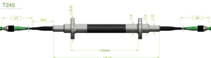
**Ready to be daisy-chained.** Well suited for projects that include the need to monitor strain at one or many locations. Provided as single sensors or in ready to install arrays of various lengths and with a flexible number of sensors. The interconnections between adjacent sensors in the arrays can be via rugged waterproof connectors (T960) or by rugged waterproof splices (T970).
