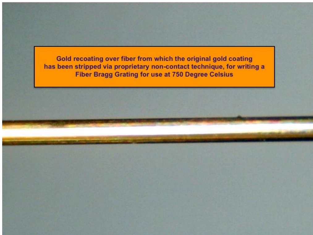
Fig.1 Schematic of a gold-coated FBG
