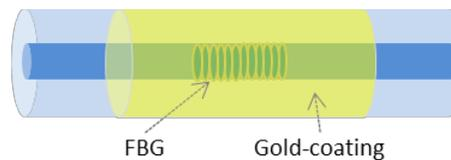
Fig.1 Schematic of a gold-coated FBG
