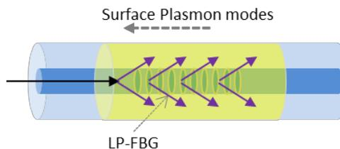
Fig. 3(b) Gold-coated Long-Period-FBG. The arrows in purple color represent cladding modes.
